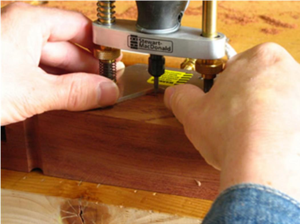
Step 4. Pictures 5 and 6 show the routed groove. Now we just have to chisel out the outside corner to make it 90° and then they are ready to take the stringing inlay.
