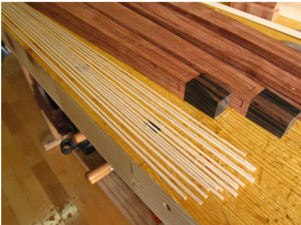
Step 6. Picture 8 and 9 show my method for cutting the mitered strings to length. I am using a 45° shoulder square and scary sharp chisel. This way I am able to make the smallest cut if I need to trim.
