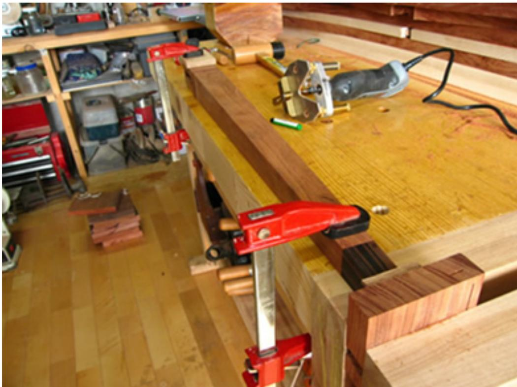
Step 3. Picture 4 shows the routing. Patience and a steady hand make this task a little less nervous. A little beeswax on the underside of the router base also helps.
